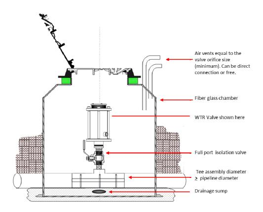
For more information on pre-assembled "drop in" fiberglass valve chambers with Vent-Tech Valves, see <a href="https://www.internationalvalve.com">www.internationalvalve.com</a>
