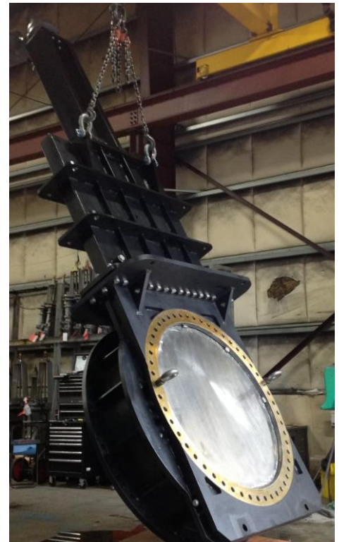
Above: Figure 193 bonneted metal seated knife gate valve with 60"x72" inlet and outlet, working in a Colorado dam.
