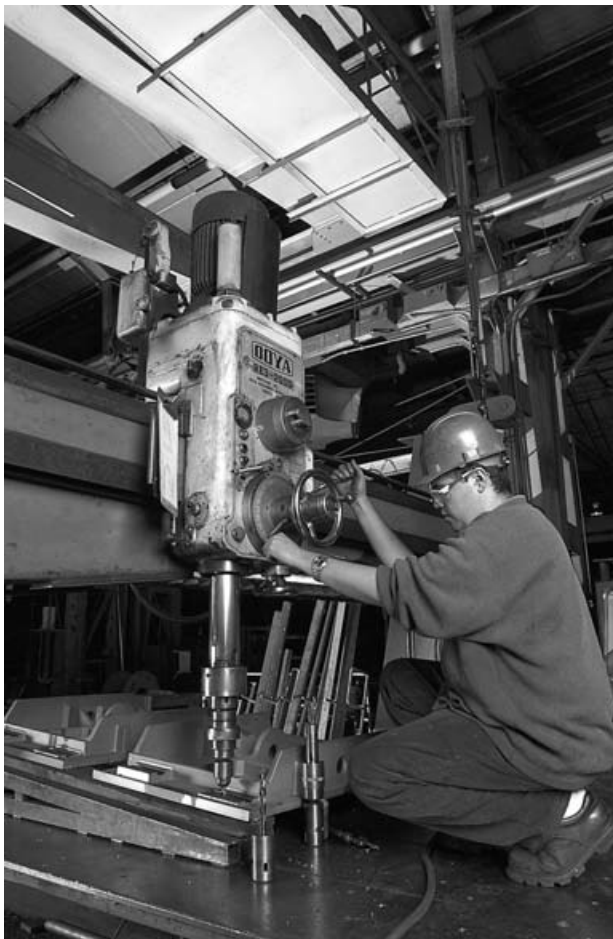
Drilling slide for wedges.
