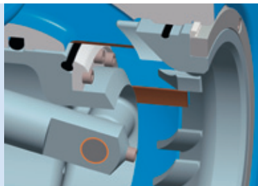
The main seal, up to 7/8 inches wide, resides on the piston periphery and recessed from direct impact of the flow media, outside the zone of cavitation and is captured in corrosion-proof stainless steel.
