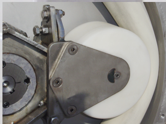
Unique roller/hose-adjustment for precise hose compression.
