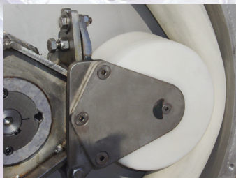
Unique roller/hose-adjustment for precise hose compression.
