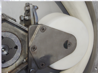
Unique roller/hose-adjustment for precise hose compression.
