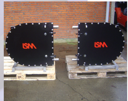
Pumps with special coatings. One pump is oriented "right" and the other "left".
