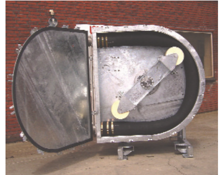
Model LSM-125 with the cover opened. The hose and fittings are the ONLY wetted part. The soft rollers, unique adjustment system and larger diameter of the rotor ensure longer hose life and lower operating costs.
