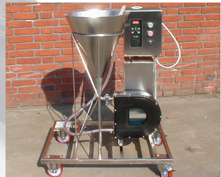
Special LSM-015 dosing unit for injection of jam into ice cream (Ghana, Africa). This design will handle many similar dosing applications, and is available tailor made for your applications.
