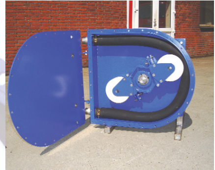
Model LSM-032 with the cover opened. The hose and fittings are the ONLY wetted part. The soft rollers, unique adjustment system and larger diameter of the rotor ensure longer hose life and lower operating costs.
