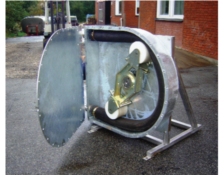
Model LSM-100 with the cover opened. The hose and fittings are the ONLY wetted part. The soft rollers, unique adjustment system and larger diameter of the rotor ensure longer hose life and lower operating costs.
