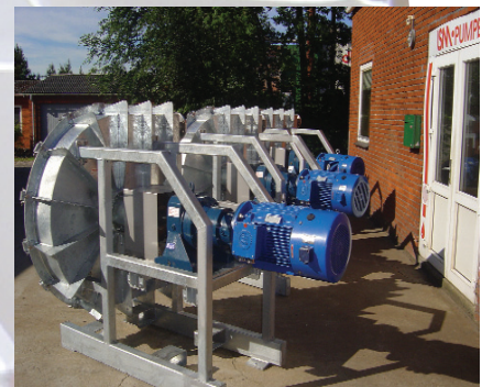
LSM-100 pumps for a mining application in Africa. The expectation to the hose life is long exceeded due to the hose quality and design of these pumps. More than Double the Hose life and Half the Power consumption than other peristaltic hose pumps.
