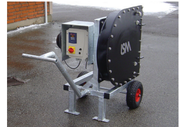
Trolley mounted LSM-025 pumping unit for manure in an agriculture facility. The pumps are reversible and are used to fill and empty a reservoir – even with fluids as Lime slurries, manure or Biomass.
