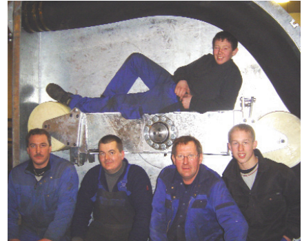
Model LSM-200 with the cover opened. The hose and fittings are the ONLY wetted part. The soft rollers, unique adjustment system and larger diameter of the rotor ensure longer hose life and lower operating costs.
