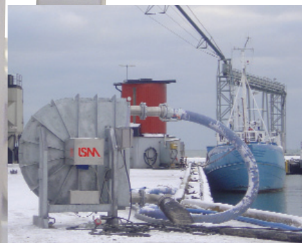
LSM-150 as an unloading facility for sea going fishing vessels. The pump is moveable and can serve different vessels. Pump materials suitable for the high humidity and salt content of the surrounding environment.
