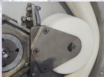
Unique roller/hose-adjustment for precise hose compression.
