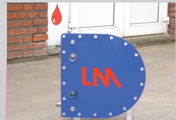
LM32 "Low Maintenance" pump. LSM "Low Simplified Maintenance" design will supersede the LM series.
