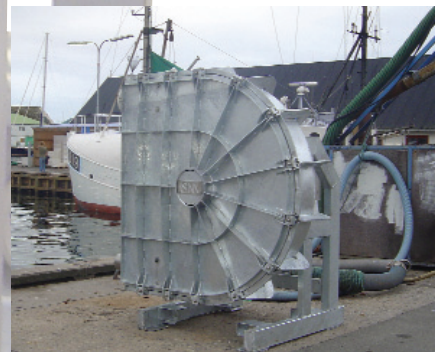
LSM-125 in an unloading facility for sea food. The LSM-series is widely used in the fishing industry as this pump design will transport the sea food without any damage to the meat. LSM can pump live fish in fish farms.
