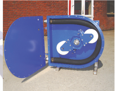
Model LSM-025 with the cover opened. The hose and fittings are the ONLY wetted part. The soft rollers, unique adjustment system and larger diameter of the rotor ensure longer hose life and lower operating costs.
