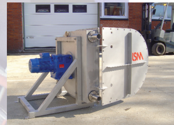
Pump housing in Stainless Steel for vacuum application in Chemical Industry. The hinged door is reinforced and with sensor holes for transmitters.
