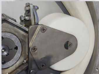
Unique roller/hose-adjustment for precise hose compression.
