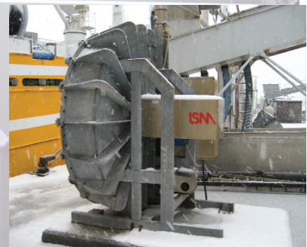
LSM-200 which replace LSM-150 as the Worlds Largest Peristaltic Hose Pump . Peak capacity in excess of 300 m 3 or 80,000 gal water per hour.
