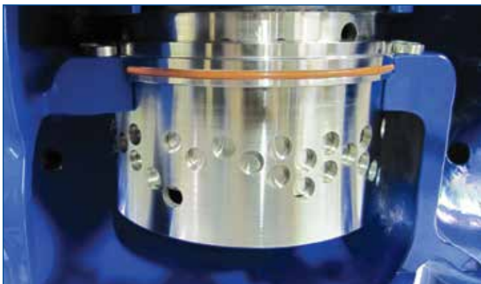
Anti-Cavitation Cages in Valve Body
