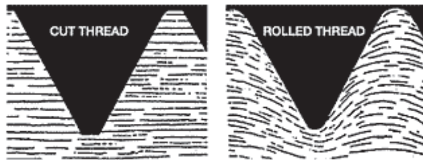
Caption: An illustration of cut thread and rolled thread – notice how the grain of the cut thread is split, but the grain of the rolled thread is a continuous line.
